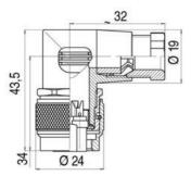
M16 Female connector - DIN For C-connection (8-Pins) Ø of the cable: 4 to 6 mm Ref: 5100-008
