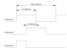
$\begin{array}{l} \mbox{Period}: 360^\circ \mbox{ (electrical)} \\ \mbox{Duty cycle}: 180^\circ \pm 10\% \\ \mbox{Phase shift}: 90^\circ \pm 25\% \\ \mbox{Starting time}: less than 100ms \end{array}$
